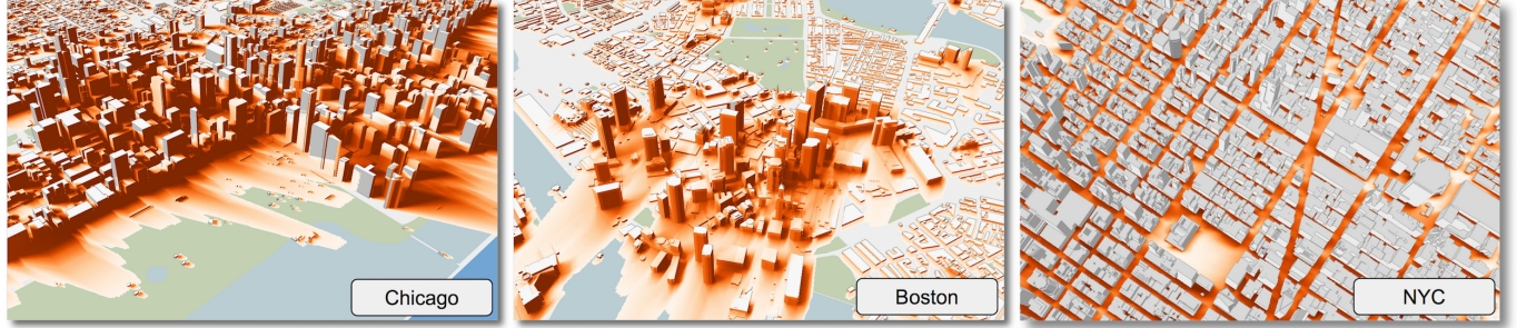
Fig. 10. Shadow profiler supports two modes of operation. The exploration mode, which uses shadow accrual maps to compute shadow accumulation, is used to explore Chicago and Boston. The analysis mode, which uses inverse accrual maps, is used for New York City. The shadows were accumulated for 7 hours on March 28.
