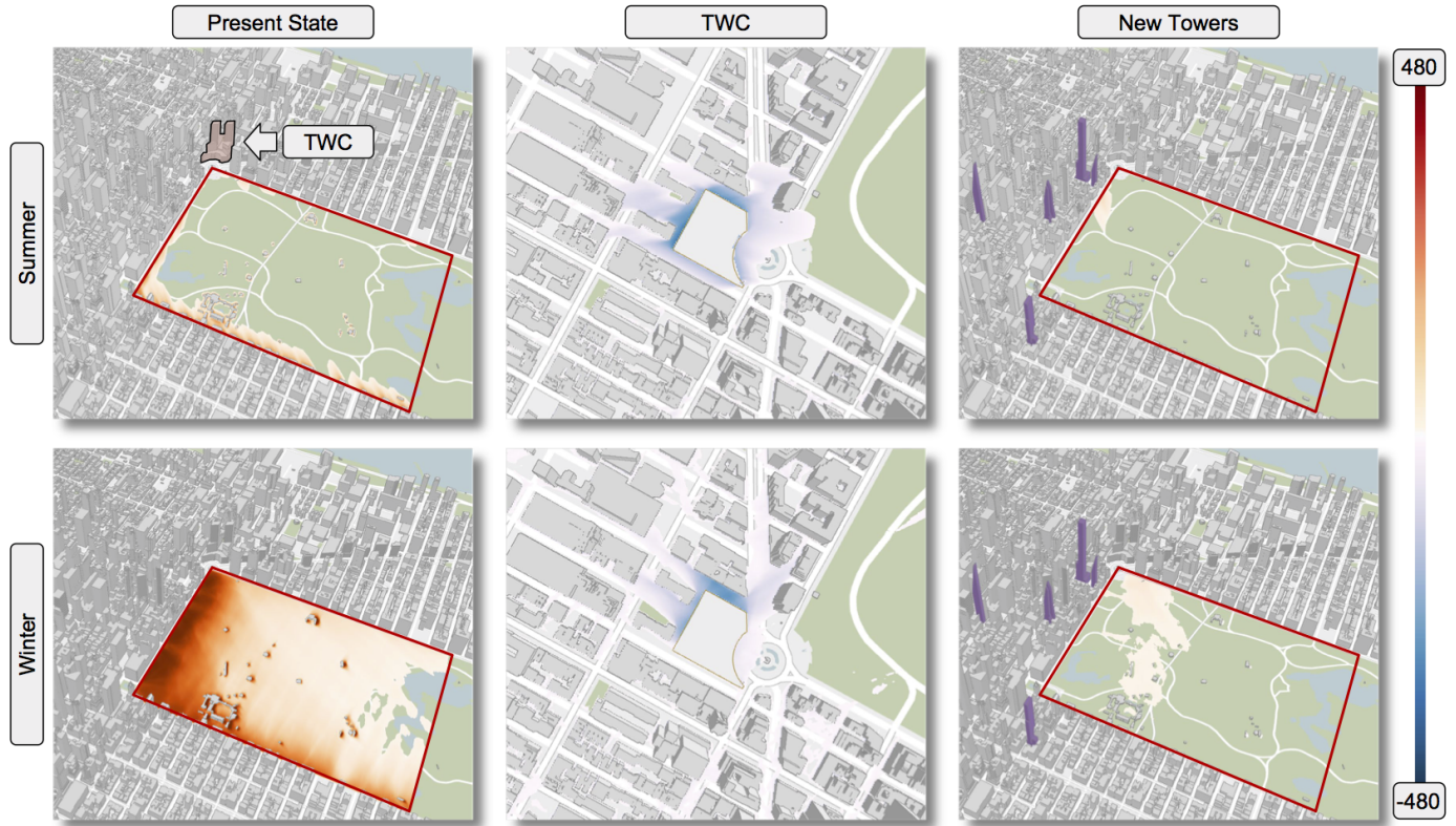
Fig. 13. Testing the impact of skyscrapers that are under construction south of Central park. Shadows cast during summer and winter with the current state (left). The impact of Time Warner Center (TWC) is used as a baseline for comparison (middle). The impact of the new towers (right). Here, we are visualizing only regions having an impact (positive as well as negative) greater than 30 minutes.
