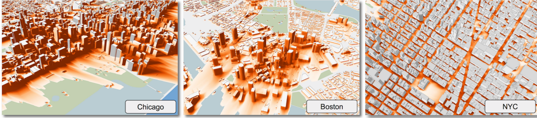
Figure 4.10: Shadow profiler supports two modes of operation. The exploration mode, which uses shadow accrual maps to compute shadow accumulation, is used to explore Chicago and Boston. The analysis mode, which uses inverse accrual maps, is used for New York City. The shadows were accumulated for 7 hours on March 28.
