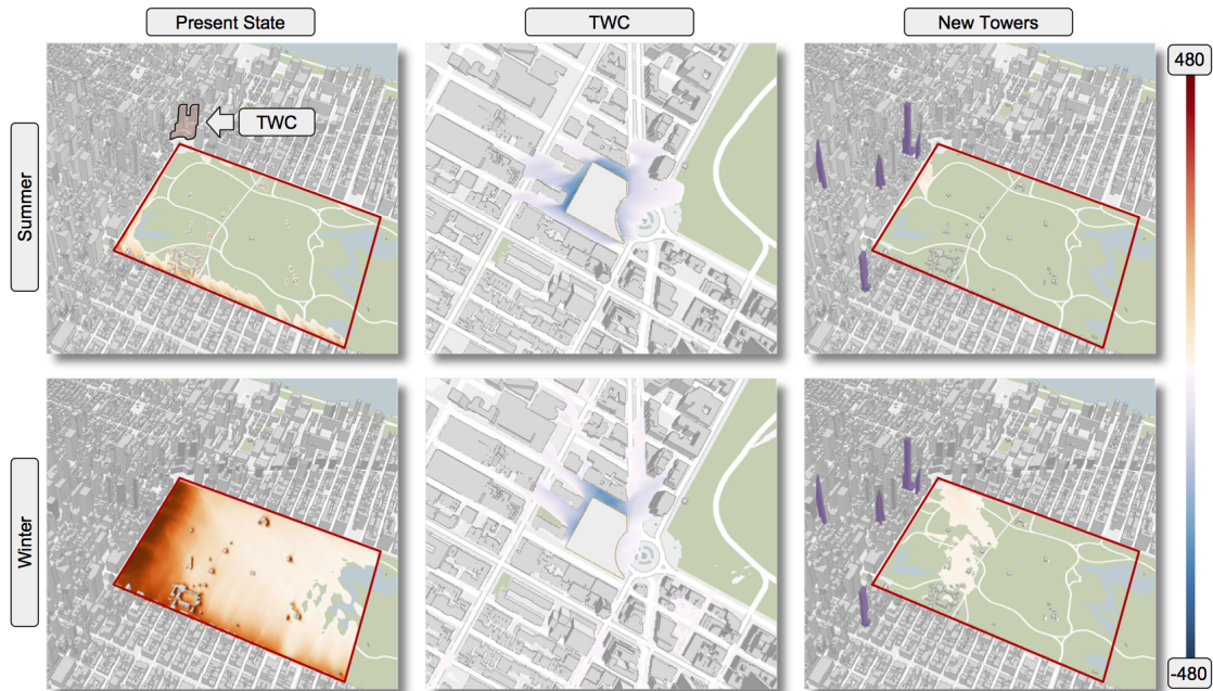
Figure 4.13: Testing the impact of skyscrapers that are under construction south of Central park. Shadows cast during summer and winter with the current state (left). The impact of Time Warner Center (TWC) is used as a baseline for comparison (middle). The impact of the new towers (right). Here, we are visualizing only regions having an impact (positive as well as negative) greater than 30 minutes.
