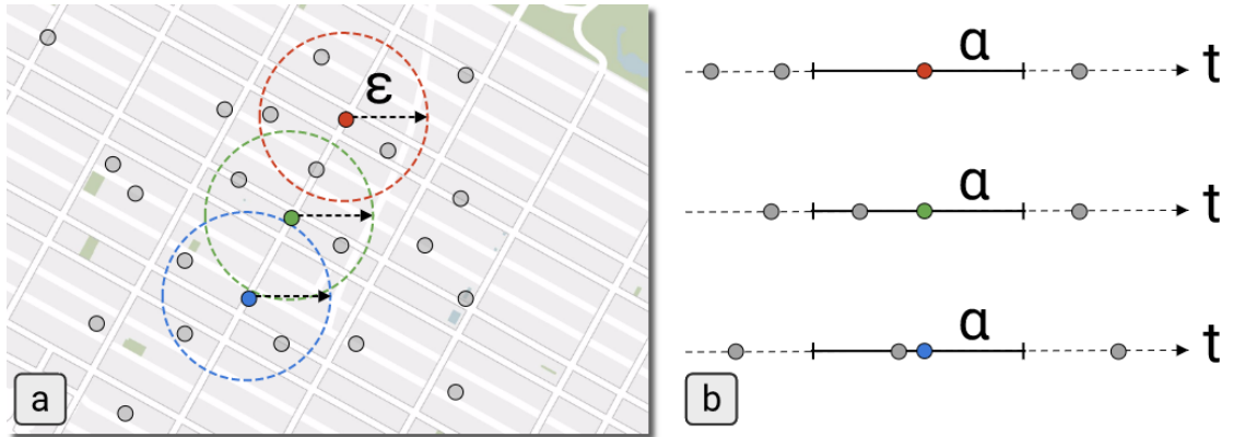
Figure 5.5: Joining images (red, green and blue dots) and urban data (gray dots). For each image, we associate the data within \epsilon meters (a) and within \alpha hours (b).
