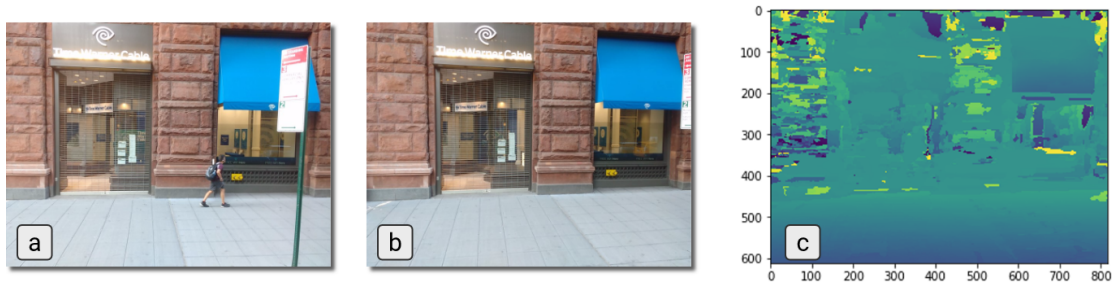
Figure 5.6: PatchMatch when considering two consecutive images ((a) and (b)). (c) shows the result, with the distance between patches.
