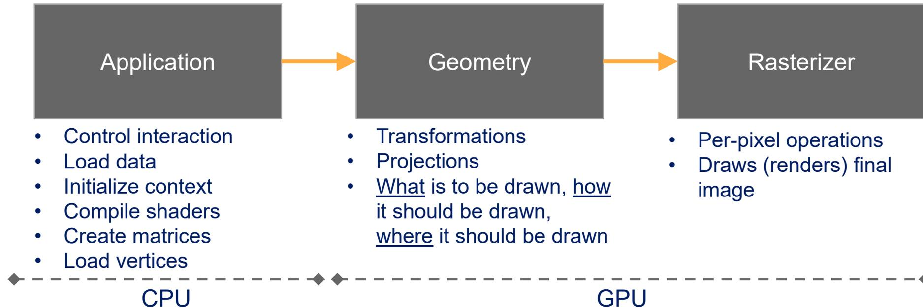
Slowest pipeline stage will determine *rendering speed* (in frames per second).
